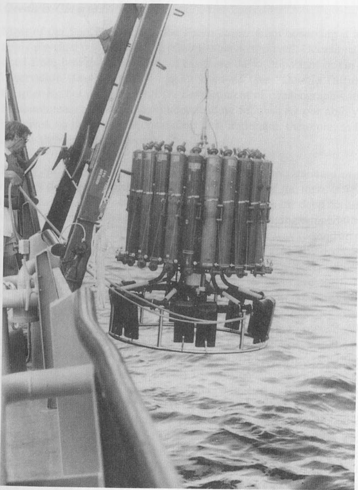
Figure 1.15 A conductivity-salinity-depth recorder (CTD) attached to a rosette sampler. The CTD records temperature and depth continuously. The rosette sampler is activated electronically from the surface and collects discrete water samples at different depths. (Photo courtesy of Thomas H. Rossby)
